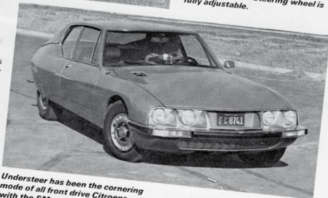
This view lets the secret out of the bag: It's a Citroën. Narrowed rear tread gives characteristic snakehipped look.
