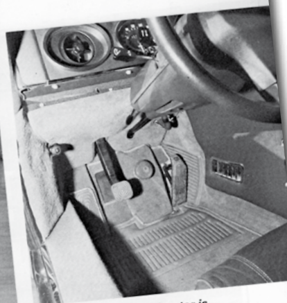
Button to left of accelerator is brake pedal. Pedal-like object to left of clutch pedal is a rest for the left foot.
