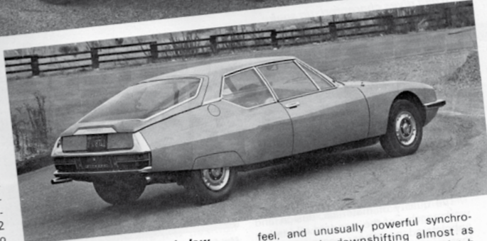
Large rear greenhouse window comes standard with heating grid to control misting problem. Rear quarter windows swing out; fronts operate electrically; front vents are immobile.
