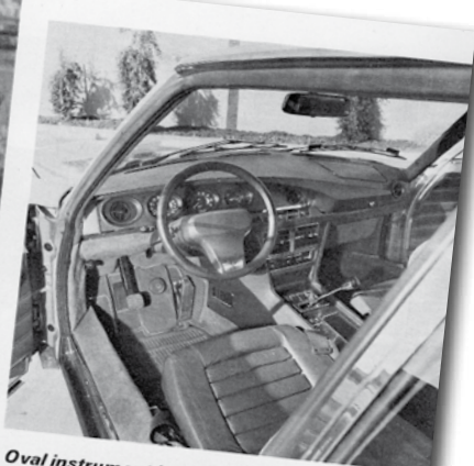
Oval instrument bezels match oval 1-spoke wheel. Control stalks on steering column, marked with symbols on European model shown here, are marked in English on U.S. version. Steering wheel is fully adjustable.
