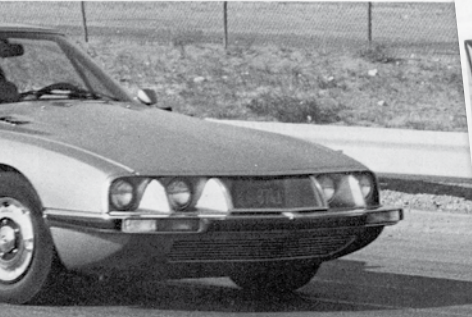
Ups and downs of hydropneumatic suspension, controlled with lever beside driver's seat, can be in 5 positions, with extreme ones used in jacking.
