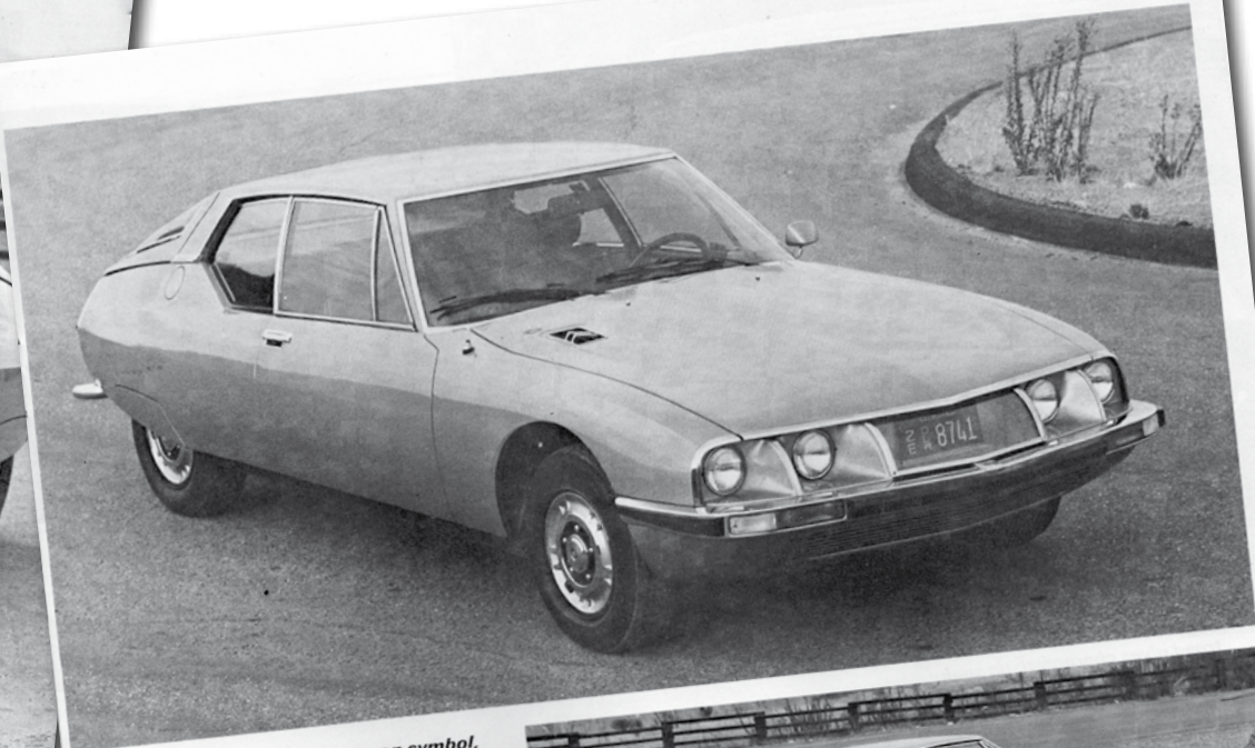
Citroën's double chevron symbol, displayed at right rear of hood, also serves as grille for heater/air conditioner fresh air intake.
